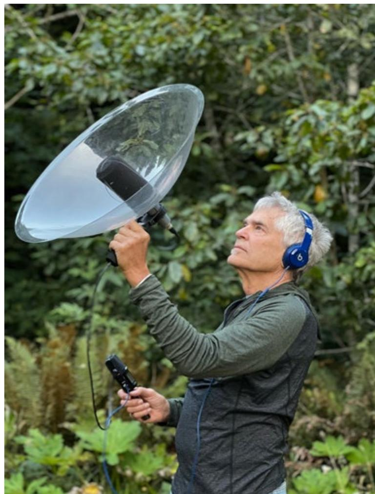
Above: The parabolic dish focuses the sound waves onto the tip of the microphone, and the recorder/amp processes and stores the signal with a time stamp.
